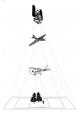
Each scene is composed of cells that determine the spatial resolution of an image. The oscillation of the scanning mirror across the scene directs the received energy to the detectors, where it is converted into electrical signals. These signals are further converted into numerical values called Digital Number (DNValues) for recording on a magnetic tape.
